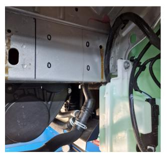
Make sure the mounting plate didn't shift during marking, you can check this by measuring the holes from the bottom of the chassis. Make sure they are on the same height measured from the bottom of the chassis.
