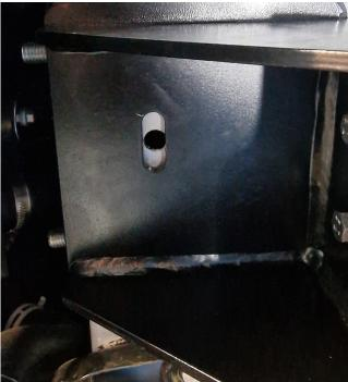
Now the bottom part needs to be secured on the chassis. Drill an 10mm (0,395 inch) hole in the bottom of the chassis.
