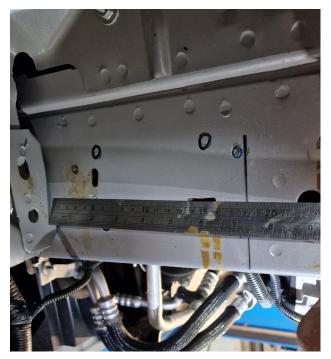
Make sure the mounting plate didn't shift during marking, you can check this by measuring the holes from the bottom of the chassis. Make sure they are on the same height measured from the bottom of the chassis.
