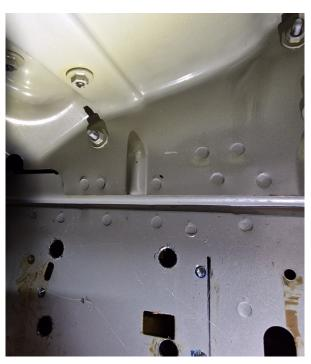
Before mounting the front mounting plate, there is a thread from the chassis that needs to be removed. Cut the thread as shown in the picture above, make sure to paint or use anti-corrosion filler so the blank metal won't rust.
