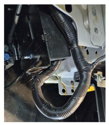
Make sure the cables are fastened as well, use tie-wraps to make sure all the cables are placed sturdy and don't hang loose.
