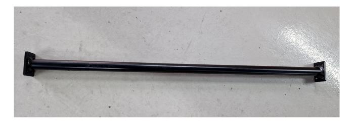
As mentioned in the main manual, if the jacks have more than 1/3rd below the chassis, there needs be a cross mount. For Ford a cross mount is neccesary, because it is impossible to have 2/3rd of the jack on the chassis height.
