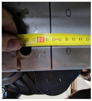
Use a tape measure to make sure the line is roughly on the same position as shown. From the corner measure around 18,5cm / 7,28 inch, and place a straight line. Position the bracket on the line and make sure the mounting plate is firmly positioned against the bottom of the chassis. Mark the four mounting holes.
