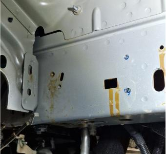
Remove the module with the bracket. The module will be placed behind the light module, as shown on the next page. The module isn't fixed with bolts so you need to drill away the metal plugs, you only need to drill away the two plugs in the chassis. As shown above with a yellow arrow.
