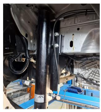
Some vehicles have a ground wire under the chassis, which can be in the way for mounting the jack. If this is the case relocate the ground wire, and make sure it has a good connection.
