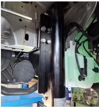
We will now use the **Mounting Plate - Bracket Font** we placed in the chassis to fix the bottom of the mounting plate to the chassis. Use the M10 x 30 Bolt together with the spring washer. If the bracket is not fully against the bottom of the chassis, loosen the 4 M12 locknuts and first tighten the bottom.
