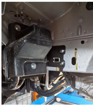
If you haven't removed the front left wheel yet, please do. Unscrew parts of the wheel arch cover and bend it back as shown in the picture above. If the vehicle got an automatic gearbox, the gearbox module will be in the way. This module needs to be relocated.
