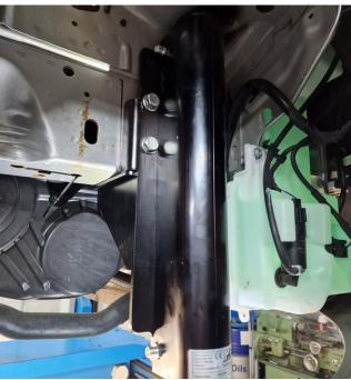
Before we can fix the mounting plate against the chassis. Make sure the jack is pre-assembled on the mounting plate. Use at least 12 M8 x 20 bolts per jack, make sure the bolts are divided over the whole jack. Make sure the hydraulic connections are facing the right way, see picture above. Fix the mounting plate on the chassis with the four M12 x 160 Bolts, M12 Rings and the M12 Locknuts. Make sure the mounting plate is placed against the bottom of the chassis.
