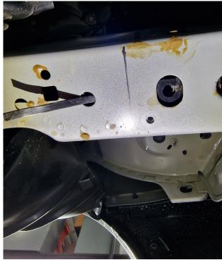
Before mounting the plate to the chassis, first place the **Mounting Plate - Bracket Font** in the chassis as shown in the picture above. Use the lager hole in the chassis to put the plate into it.
