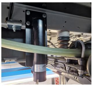
The rear jacks will be mounted close behind the wheels. The closer the jack can be placed to the wheel, the lower it can be installed without causing problems. We always advice a minimum height clearance to the floor of 15-17cm (6-7 inch).
