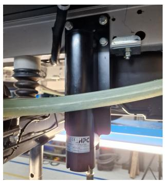
Do the same for the other side if you haven't already. Check if the hydraulic connections face the correct way and make sure all the bolts and nuts are tightened accordingly.
