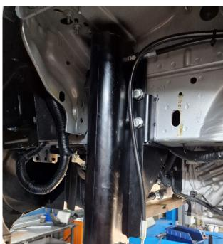
We will now use the **Mounting Plate - Bracket Font** we placed in the chassis to fix the bottom of the mounting plate to the chassis. Use the M10 x 30 Bolt together with the spring washer. If the bracket is not fully against the bottom of the chassis, loosen the 4 M12 locknuts and first tighten the bottom.
