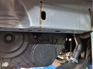
Remove the protective cover as shown in the picture above, so the bracket can be mounted against the bottom of the chassis. Before we can position the mounting plate we need to remove parts of the tank shown below. The two lips that hold the cable need to be removed.
