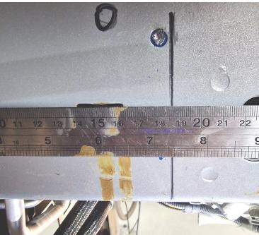
We will now start mounting the left mounting plate, this will be the same as the right side. Use a tape measure or a ruler. From the corner measure around 18,5cm / 7,28 inch, and place a straight line. Position the bracket on the line and make sure the mounting plate is firmly positioned against the bottom of the chassis. Mark the four mounting holes.
