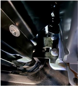
Remove the two bolts shown in the picture above. The top hole needs the be a slot to make the module with bracket fit. Adjust the hole and mount the module with the two original bolts.
