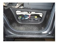
Situation where the battery box is located under the driver's seat.
