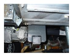
The battery box is placed at the same height as the stabilization bar which requires the bracket to be placed in front of or behind the stabilization bar.
