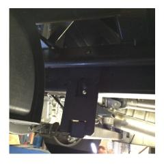
Example of removing the battery box under the driver's seat.
