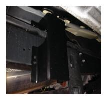
Example where the mounting plate is placed in front of the stabilization bar.
