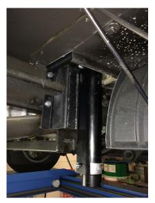
Example of removing the battery box and placing the mounting plate over the stabilization bar.
