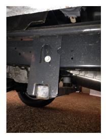
Example where the mounting plate is placed over the stabilization bar.
