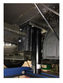
In almost all cases the mounting plate can be placed over the stabilization bar.
