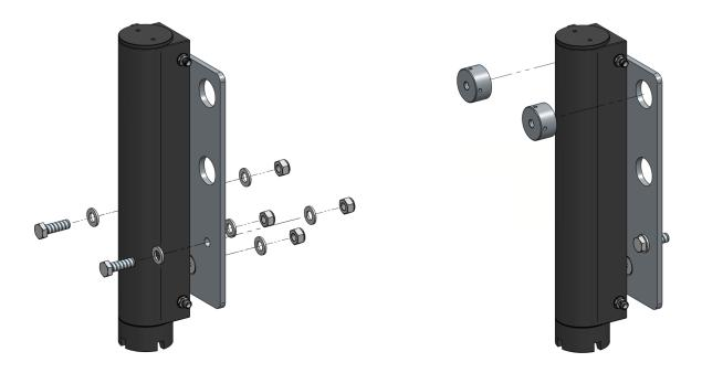
Place the stabilizing bar between the mounting plates and attach it where the holes are drilled. Fasten the stabilizing bar with six-side bolts M8 x 25 and springwashers. (If for some reason this is not possible, use a small amount loctite so that the bolts can be looseended later without causing damage.)
