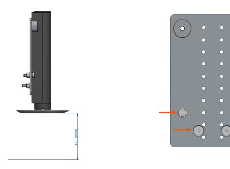
Temporarily mount the mounting plate with the M12 bolts. This makes it easy to determine the height. Take into account the foot that has yet to be placed. Allow 1 centimeter extra for this.
