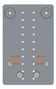
Disassemble the mounting plate after the holes have been drilled. Mount the jack at the correct height and fix it with the 10 countersunk bolts M8 x 20 supplied. Position the bolts so that the jack is secured in as many positions as possible. See right image below.
